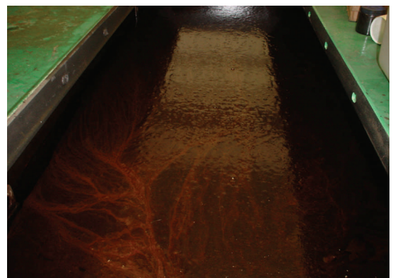
Coal tar in separator. Coal tar consistency can vary as it is recovered. The system was designed to accommodate changes in coal tar.
